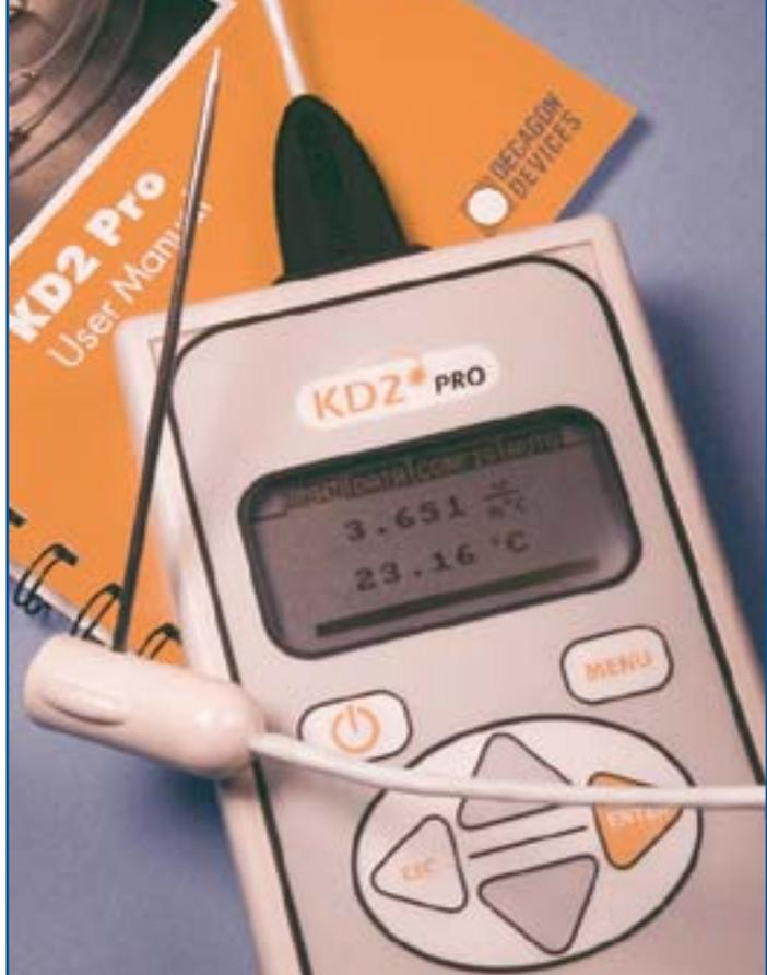
▲ In addition to thermal conductivity and thermal resistivity, the new KD2 Pro measures thermal diffusivity and specific heat (heat capacity).
