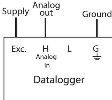
If your MPS-1 is equipped with the standard 3.5mm plug, and you wish to connect it to a non-Decagon datalogger, you have two options. First, you can clip off the plug on the sensor cable, strip and tin the wires, and wire it directly into the datalogger. This has the advantage of creating a direct connection with no chance of the sensor becoming un-plugged; however, it then cannot be used in the future with a Decagon Em50 or Em50R logger.
