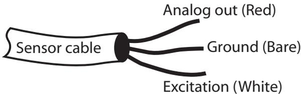
MPS-1 sensors with stripped and tinned cable option can be made with custom cable lengths up to 50ft (15m) on a per foot fee basis. This option gets around the need for splicing cables.
