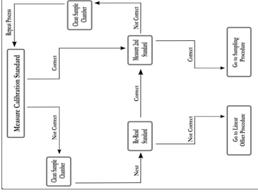
*This flowchart is a graphical representation of the directions given above for checking for linear offset.*
