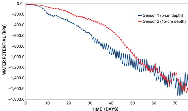
Figure 8 Temperature sensitivity data for TEROS 21 sensors
