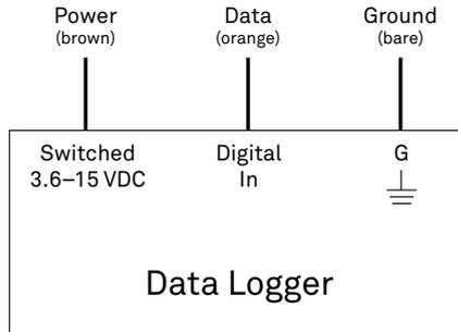
**Figure 3 Wiring diagram**
