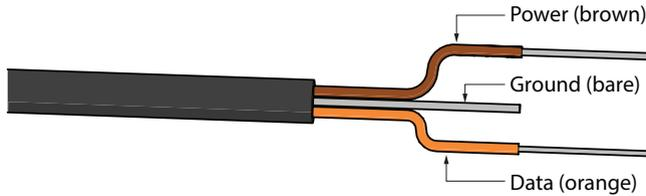
**Figure 2 Pigtail wiring**
