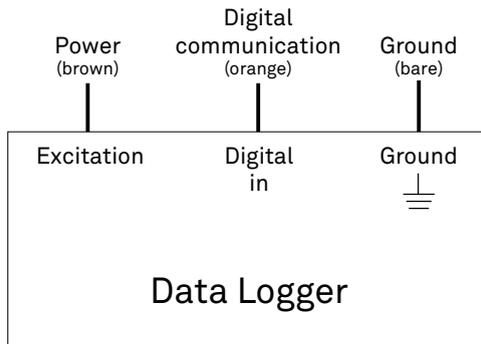
Figure 3 Wiring diagram
