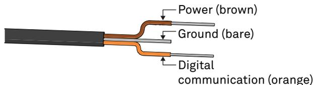
**Figure 2** Pigtail wiring
