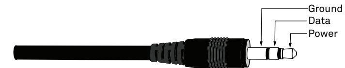
Figure 1 3.5 mm stereo plug wiring
