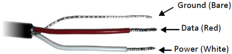
Figure 2: Pigtail End Wiring
