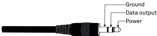
Figure 2 Stereo plug connector
