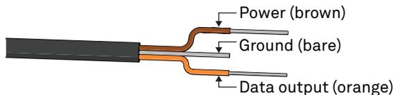
Figure 3 Pigtail wiring
