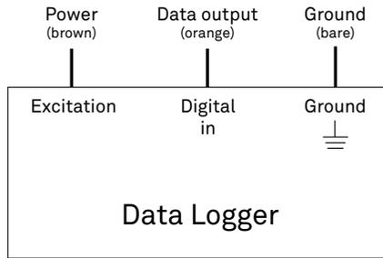
Figure 4 Wiring diagram
