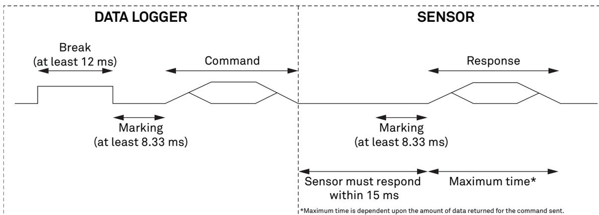
Figure 5 Example data logger and sensor communication
