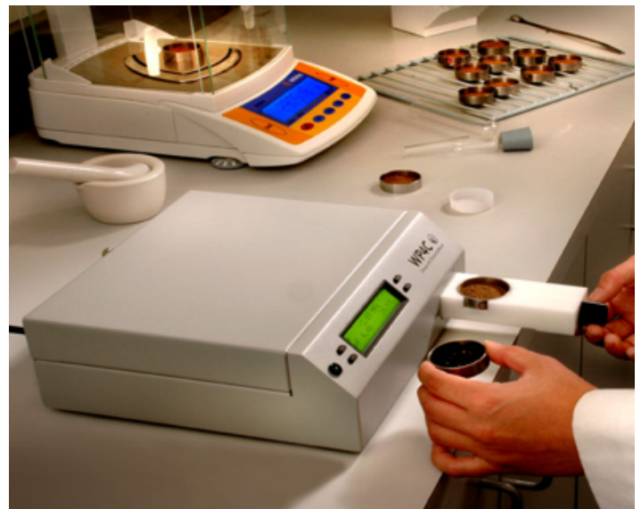
The WP4C determines water potential by measuring the temperature of the sample and the dew point of the air in a sealed head space.
