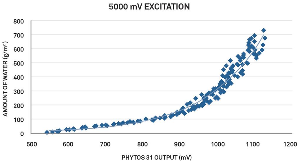
Figure 3 Amount of water on the PHYTOS 31 surface as a function of the PHYTOS #1 mV output when excited at 5000 mV
