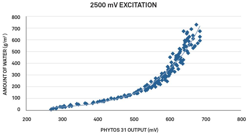
Figure 2 Amount of water( $\text{g}/\text{m}^2$ ) on the PHYTOS 31 surface as a function of the PHYTOS 31 mV output when excited at 2500 mV
