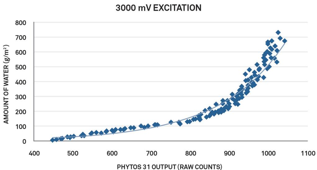
Figure 1 Amount of water(g/m<sup>2</sup>) on the PHYTOS 31 surface as a function of PHYTOS 31 raw counts measured with METER Em50 series data logger
