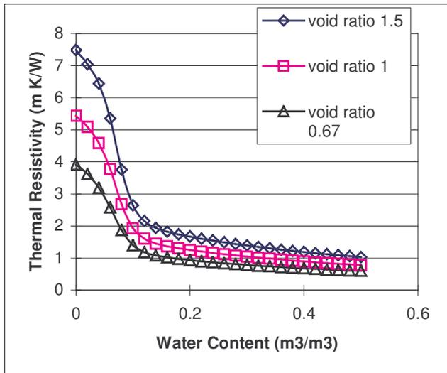
**Figure 2** Effect of density and water content on thermal resistivity of a loam soil. The void ratio 1 curve is the same as in Fig. 1. The bulk densities are 1.06 Mg/m<sup>3</sup> for void ratio of 1.5, 1.33 Mg/m<sup>3</sup> for void ratio 1, and 1.59 Mg/m<sup>3</sup> for void ratio of 0.67.
