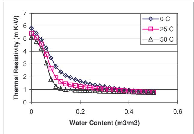
**Figure 3** Effect of temperature and water content on thermal resistivity of a loam soil. The 25 C curve is the same as in Fig. 1.
